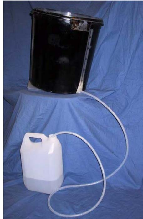
*Another way to increase speed is to dome shape the lid on the fermenting vessel with a hot air gun. That way you can keep the false bottom and don't have to tilt the vessel. Takes some skill though to shape it.*
