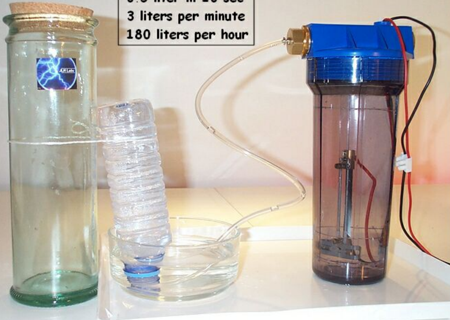
The BingoFuel Reactor - Gas output measurement by Jean-Louis Naudin (c) 2003 JL Naudin - 04-03-03 - Email: Jnaudin509@aol.com - http://www.jlnlabs.org
